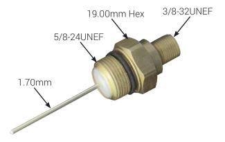
Special purpose adapter intended for situations where hardline (500) coax needs conversion down to RG-6 or similar reduced diameter drop cable. The reduced diameter end has a standard  $3/8 \times 32$ UNEF thread. The larger hardline thread is a  $5/8 \times 24$ UNEF.
